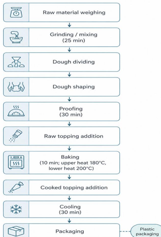
Figure 2. Production flow diagram for bread at Home-Based Food Industry “X” in Banjarbaru
